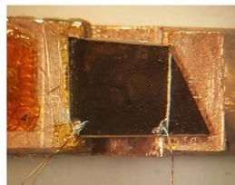
➤ A photograph of sample C with thermocouples attached. The heater is seen on the left side
